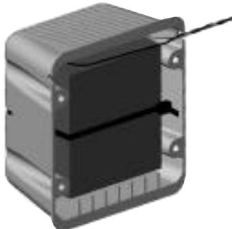
Use 4, 3/4 inch(19mm), #10 pan-head sheet metal screws to fasten the battery box to the wall.
