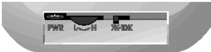
Left to right: 12vAC power jack, signal field adjustment knob, 7KHz-10KHz channel switch.
