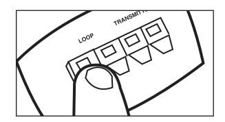
Insert the ends of the two transmitter wires into the right two black connector holes on the bottom of the LP-4100 (and side if LP-4200).
