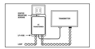
If you have added the LP-4100/4200 to an existing containment system, check the signal field for width and continuity. Adjust as necessary. If the LP-4100/4200 is being installed with a new system, follow the signal field adjustment procedures given in the containment system's owner's guide.
